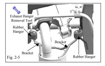
(g) Pry the two rear muffler exhaust brackets loose from the rubber hangers. (Fig 2-5)
