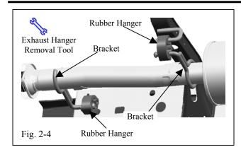
(f) Pry the two front muffler exhaust brackets loose from the rubber hangers. (Fig. 2-4)
